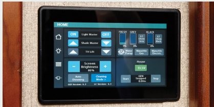
Firefly Integrations touch-screen panel provides controls for lighting, tank monitors, awning, automatic shades and TV lift.
