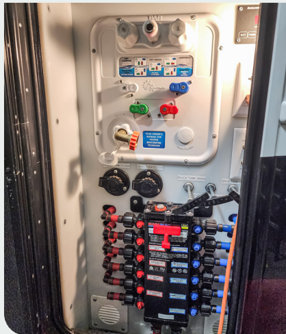
Utility center's residential manifold water system includes shut-offs for each fixture, black and gray tank flush-outs and dump valves.
