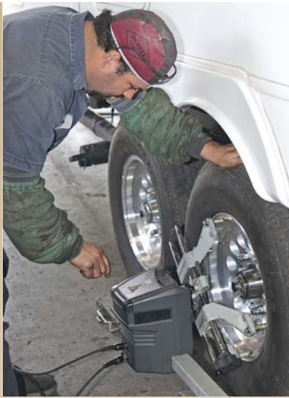
MOR/ryde uses a sophisticated laser system to ensure proper alignment.
