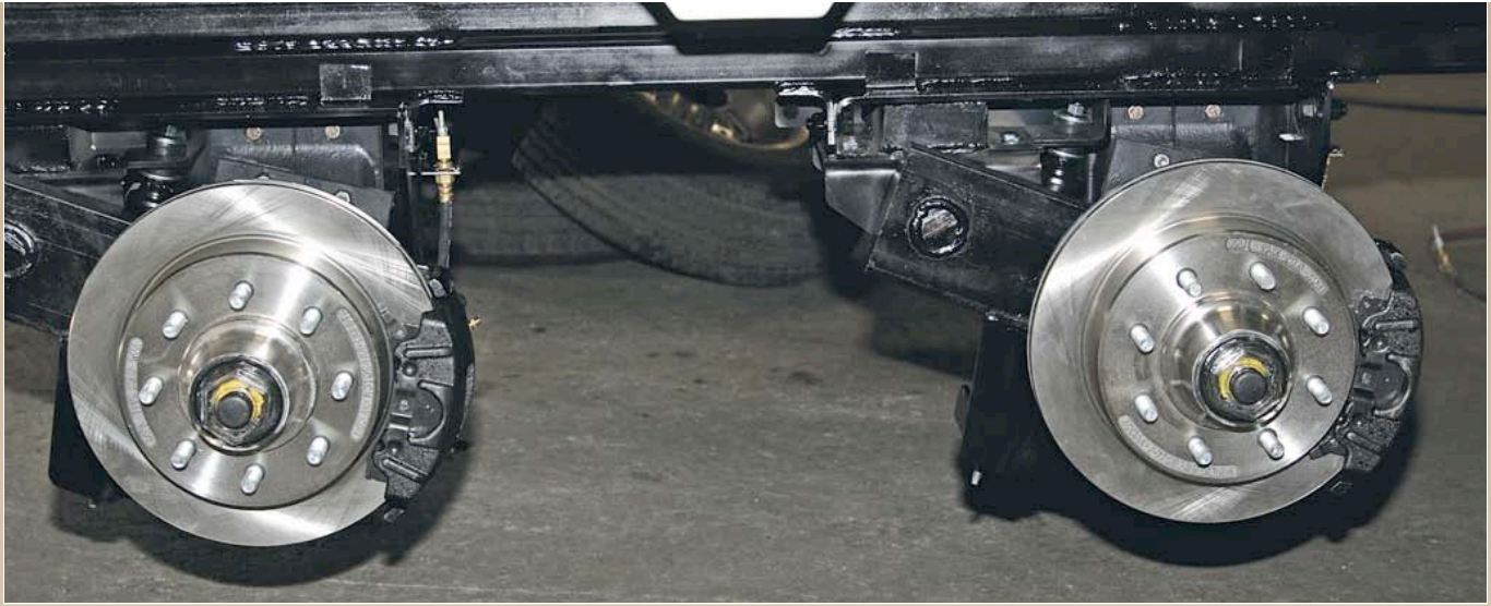
The completed MOR/ryde IS Suspension System upgrade with Kodiak Disc Brakes. Next up: tires, wheels, and laser alignment.
